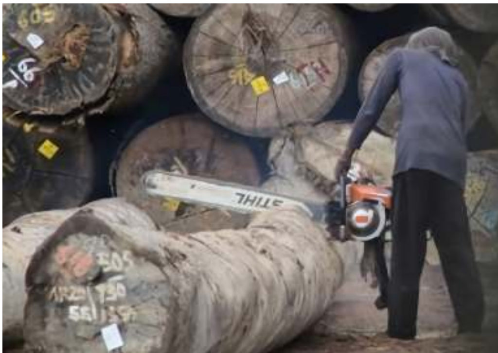
Figure 40. Worker working without proper PPEs
